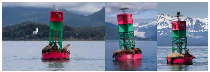
Poundstone Rock buoy (LLNR 23845) is a red and green lighted bell buoy located near the northern end of Favorite Channel at 58.528838,-134.933743 almost exactly due west of Eagle River and Herbert Glacier. It marks the location of a rock that lies only 2 fathoms (12 feet) below the water surface at mean low tide. These photos illustrate the view to its north northeast is the Sentinel Island Lighthouse, to the east the Herbert Glacier and to the west the Chilkat Mountains across the Lynn Canal.
